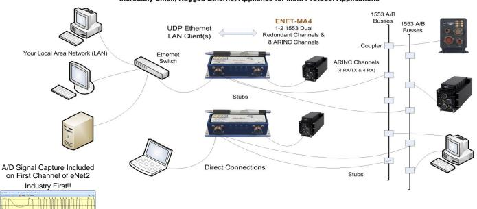
**eNet-MA4**™ is an innovative product for "remoting" 1553 & ARINC-429/717 operations on 10/100/1000 Ethernet local area networks (LAN). eNet-MA4 is a very small, low-power, rugged device that provides real-time UDP connectivity to for 1-2 dual redundant 1553 (A/B) busses and 8 ARINC channels.
